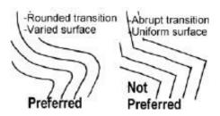
vi. Site design and grading shall establish contours and gradients that resemble the naturally occurring terrain. Site design shall round out slope transitions and blend transitions between lots or adjacent to undisturbed areas, as illustrated.
