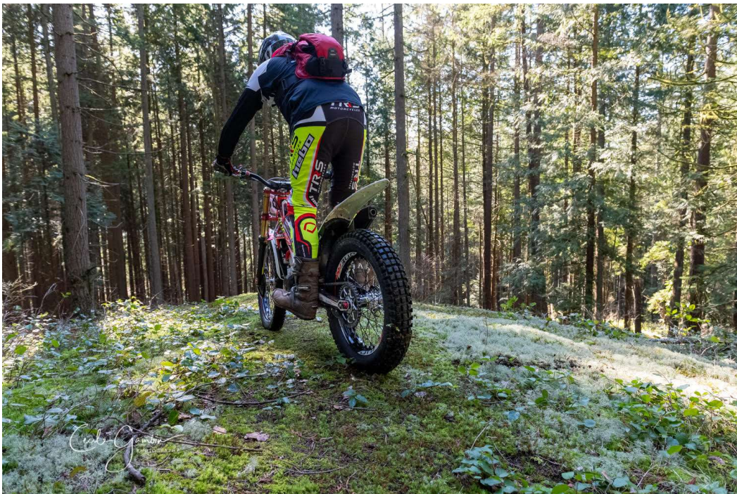
Figure 2: Low tire pressures and the soft compound of trials tires leave a very light footprint on the trail.
